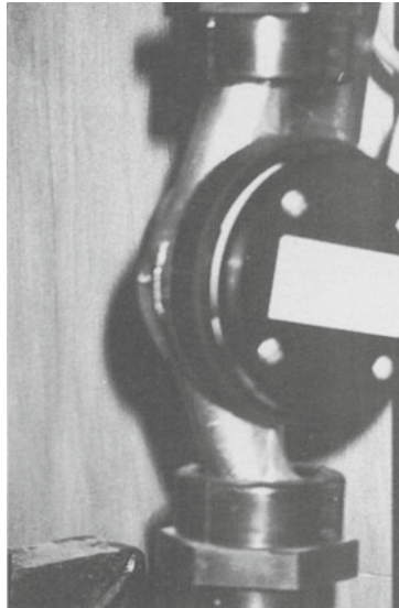
Figure 3.10 Two industrial flowmeters: (a) an electromagnetic type; and (b) a rotating impeller type. Both are on 2.5 cm pipes.
