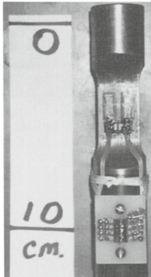
Figure 3.8 These strain gauges are mounted on a shaft to allow the measurement of shaft twist and the inference of torque.
